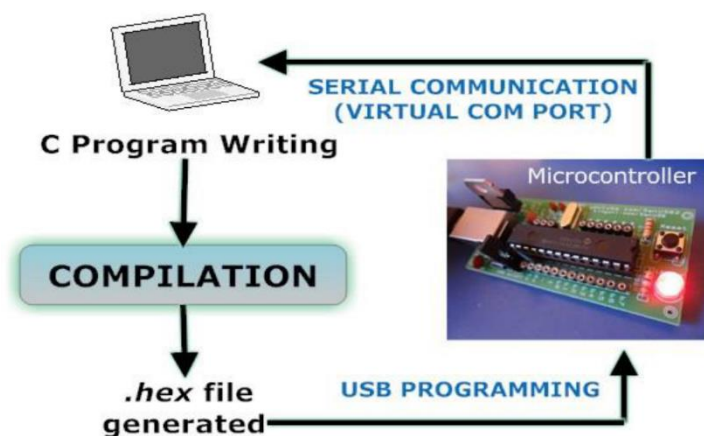
Figure 5. Recording PIC microcontroller through SanUSB [12].
